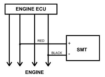
While others have to be cut and soldered onto wires supplied in the SMT harness.
